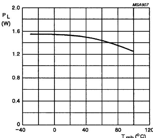
$Z_S = Z_L = 50 \Omega$ ;  $P_D = 2 \text{ mW}$ ;  $V_S = 6 \text{ V}$ ;  $V_C = 3.5 \text{ V}$ ;  $f = 890 \text{ MHz}$ .
